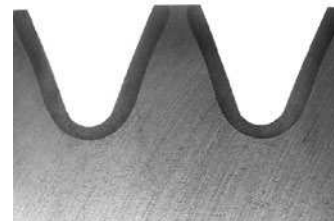
Selective Hardened Flanks and Root
